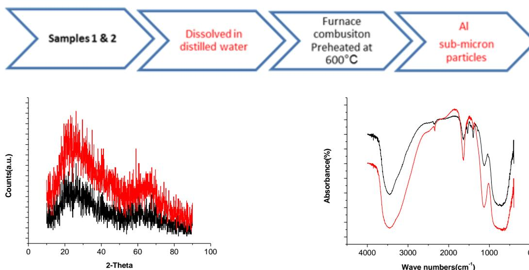
Fig.1. XRD spectrum of sample 1 and 2 at 600 ° C for 3 hours. Red (S<sub>1</sub>) and black (S<sub>2</sub>).
