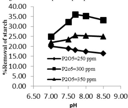
Figure 5. Effect of pH and phosphate on removal of starch.
