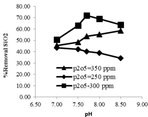
Figure 4. Effect of pH and phosphate on removal of SiO<sub>2</sub>.
