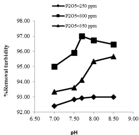
Figure 7. Effect of pH and phosphate on removal of turbidity.
