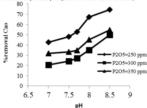
Figure 8. Effect of pH and phosphate on removal CaO.
