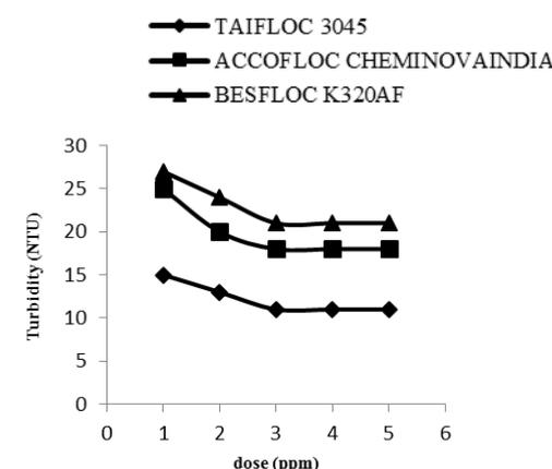
Figure 3. Effect of dose polyelectrolyte on turbidity.
