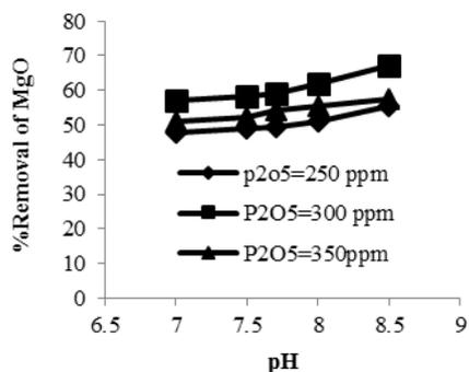
Figure 9. Effect of pH and phosphate on removal of MgO.
