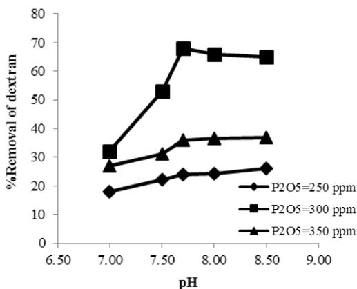
Figure 6. Effect of pH and phosphate on removal of dextran.
