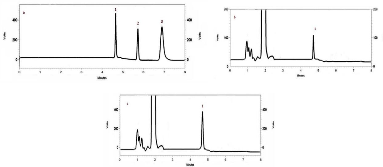
Figure 5. HPLC chromatograms of (a) standards ( $10 \mu\text{g mL}^{-1}$ ), (b) urine sample, and (c) model urine sample ( $5 \mu\text{g mL}^{-1}$  of 4-AP) after IL-SDME. Peak identification: (1) 4-AP, (2) 3-AP, (3) 2-AP
