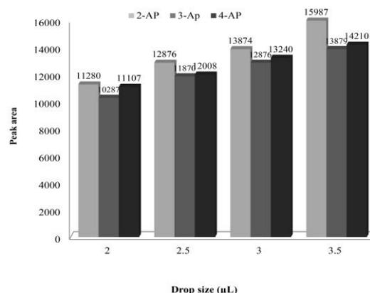
Figure 2. Effect of micro-drop volume on the extraction efficiency of Aps. Conditions: ionic liquid:  $[C_6MIM][PF_6]$ , sample 10 mL, without pH adjustment and salt addition, stirring rate: 800 rpm, extraction time: 20 min, at room temperature
