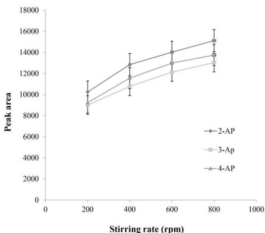
Figure 4. Effect of stirring rate on the extraction efficiency of APs Conditions: ionic liquid: 3  $\mu\text{L}$  of  $[\text{C}_6\text{MIM}][\text{PF}_6]$ , sample 10 mL, without pH adjustment and salt addition, extraction time: 15 min, at room temperature
