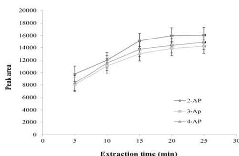
Figure 3. Effect of extraction time on the extraction efficiency of Aps. Conditions: ionic liquid: 3  $\mu$ L of  $[C_6MIM][PF_6]$ , sample 10 mL,
