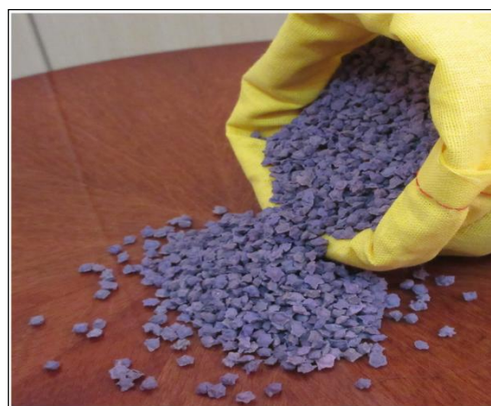
Fig. 6. The coated sugar beet seeds with synthesized copolymer (with KPS as initiator).
