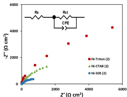
**Fig. 7.** The Nyquist diagrams recorded in 1 M NaOH solution for Ni samples electrodeposited at surfactant concentration equal to the CMC point, inset: The equivalent circuit compatible with the experimental Nyquist diagrams.
