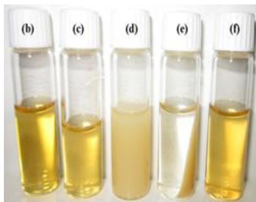
Figure 5. Photograph of (b) 2 ml of AgNPs+2 ml of DMSO, (c) 2 ml of AgNPs+1 ml of DMSO +0.3 g (\text{NH}_4)_2\text{SO}_4 , (d) 2 ml of AgNPs+1 ml of DMSO+0.3 g (\text{NH}_4)_2\text{SO}_4 +1 ml of DMSO, (e) solution (d) after centrifugation, (f) the solid phase of (e) after resuspension in 3 mL of water.
