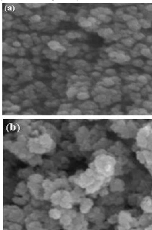
Figure 5. SEM images of (a) undoped ZnO, and (b)  $V_2O_5$ -doped ZnO ( $V/Zn=0.1$ ) nanoparticles.
