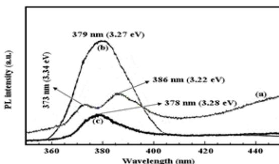
Figure 8. PL spectra of (a) undoped ZnO, (b)  $V_2O_5$ -doped ZnO ( $V/Zn=0.1$ ), and (c)  $V_2O_5$ -doped ZnO ( $V/Zn=0.15$ ) nanoparticles.
