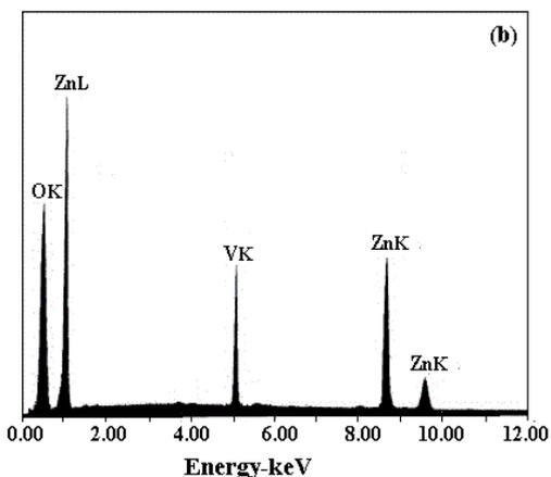
Figure 7 EDX spectra  $V_2O_5$ -doped ZnO ( $V/Zn = 0.1$ ) nanoparticles. Also, these results are consistent with the XRD and FT-IR data.
