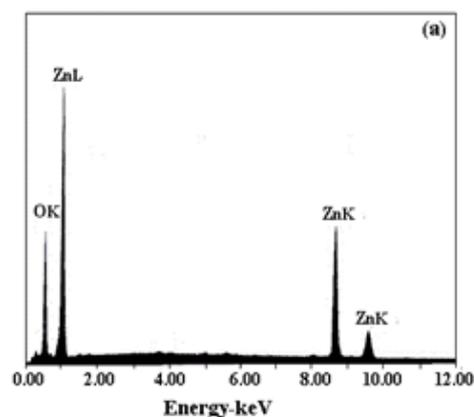
Figure 6. EDX spectra of undoped ZnO
