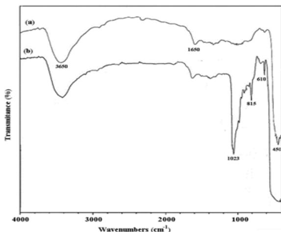
Figure 4. FT-IR spectra of (a) undoped ZnO, and (b)  $V_2O_5$ -doped ZnO ( $V/Zn = 0.1$ ) nanoparticles.
