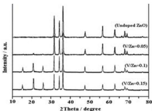
Figure 3. XRD patterns of  $V_2O_5$ -doped ZnO samples using ZnO calcined at  $750^\circ\text{C}$  temperature for 3h.
