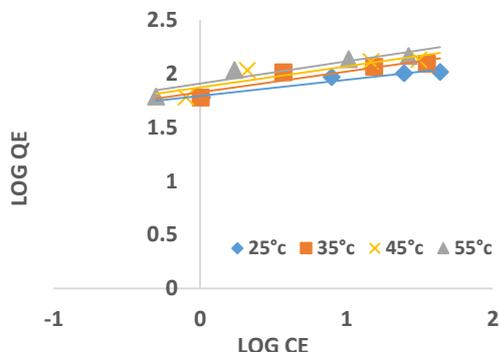
Figure 8. Freundlich plot for Direct red 81 biosorption at different temperature
