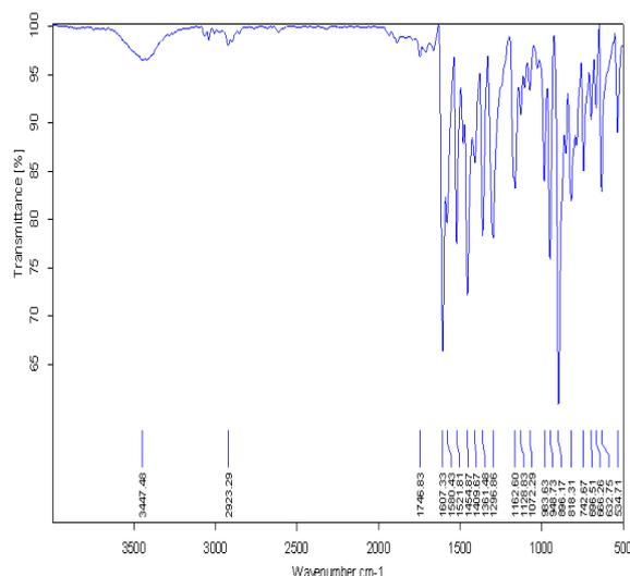
**Figure 2.** FT-IR spectrum of dioxidouranium (VI) complex  $[UO_2(L)(DMF)]$
