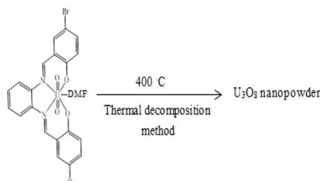
**Scheme 1.** Synthesis of nano sized U<sub>3</sub>O<sub>8</sub> and dimethyle formamide - 2, 2'-((1E, 1E')-(1, 2 phenylen bis (azanylylidene)) bis (methanylylidene)) bis (4-bromo phenolato dioxidouranium (VI) complex [UO<sub>2</sub>(L)(DMF)] as a precursor
