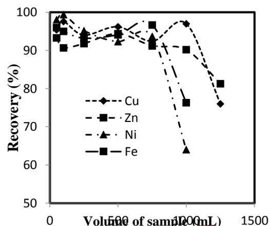
**Fig. 7.** Effect of sample volume on metal ions recoveries, pH: 7, sorbent: 0.3 g, eluent: nitric acid 4.0 mol L<sup>-1</sup>, 6.0 mL, flow rate (sample): 2.0 mL min<sup>-1</sup>.
