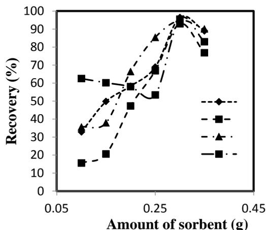
**Fig. 5.** Effect of amount of solid phase on metal ions recoveries, pH: 7.0, eluent: nitric acid, 4.0 mol L<sup>-1</sup>, 5.0 mL, flow rate (sample): 2.5 mL min<sup>-1</sup>, flow rate (eluent): 1.0 mL min<sup>-1</sup>.
