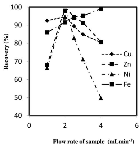
**Fig. 6.** Effect of flow rate of sample on metal ions recoveries, pH: 7, sorbent: 0.3 g, eluent: nitric acid 4.0 mol L<sup>-1</sup>, 6.0 mL, flow rate (eluent): 1.0 mL min<sup>-1</sup>.
