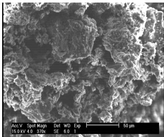
Fig. 3. SEM image of modified SWCNT.
