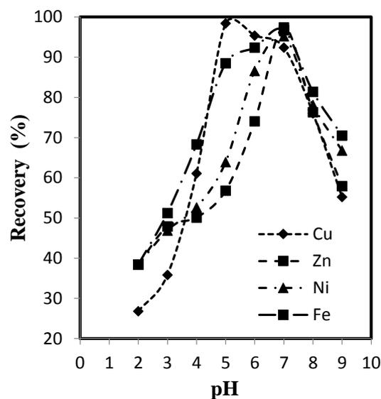
Fig. 4. Effect of pH on metal ions recoveries, sorbent: 0.2 g, eluent: nitric acid,  $4.0 \text{ mol L}^{-1}$ , 5.0 mL, flow rate (sample):  $2.5 \text{ mL min}^{-1}$ , flow rate (eluent):  $1.0 \text{ mL min}^{-1}$ .
