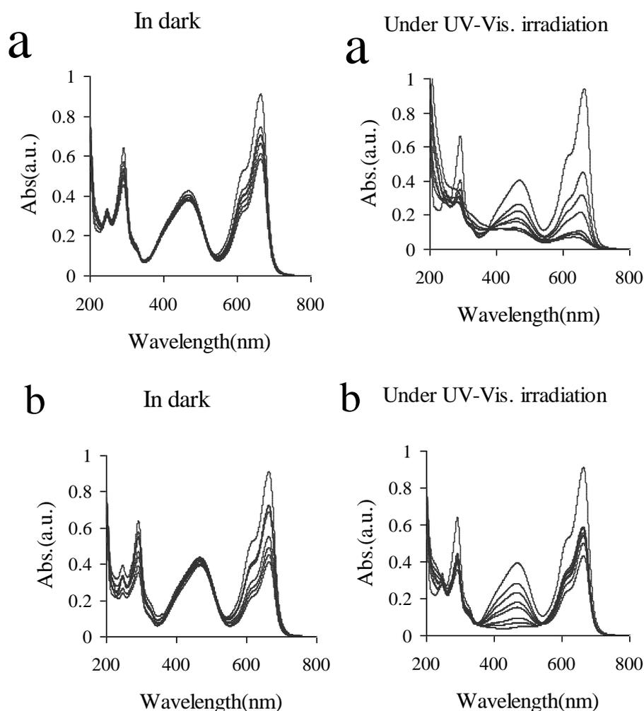
**Fig. 3.** UV-Vis. spectra changes of a two dye mixture- methylene blue (M.B.) and methyl orange (M.O.) solution in the presence of (a) amorphous and (b)  $\text{SnO}_2/\text{Zn}_2\text{SnO}_4$  samples in dark and under UV-Vis. irradiation conditions.
