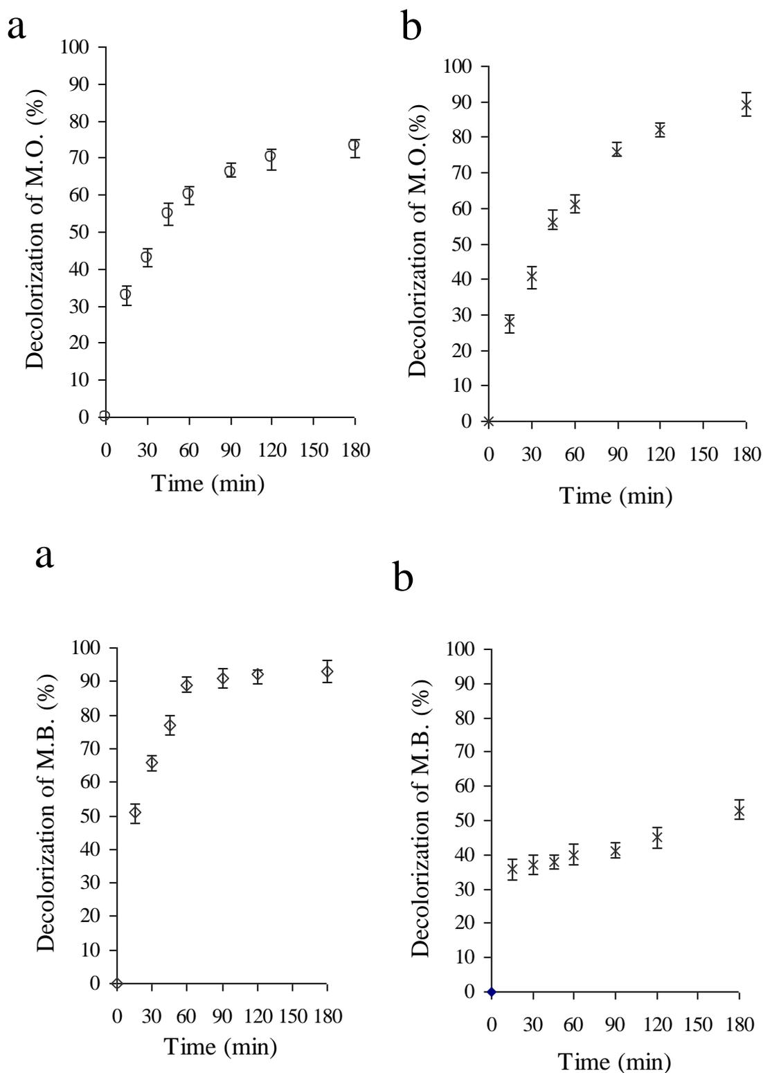
**Fig. 4.** The plots of photodecolorization percentage of two dye mixture- methylene blue (M.B.) and methyl orange (M.O.) solution versus time in the presence of (a) amorphous and (b)  $\text{SnO}_2/\text{Zn}_2\text{SnO}_4$  samples.
