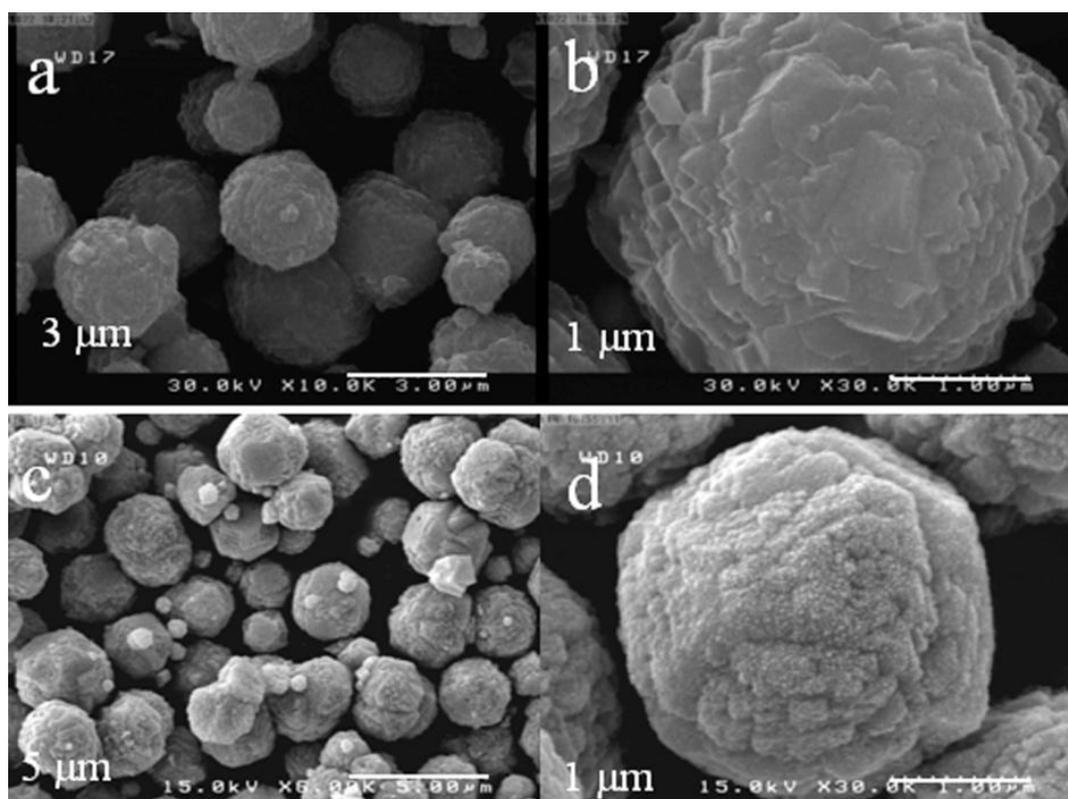
Fig. 2. The SEM images of (a, b) amorphous and (c, d) SnO<sub>2</sub>/Zn<sub>2</sub>SnO<sub>4</sub> samples.
